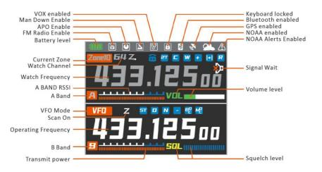
stThe highlighted band is the main channel (i.e., the working band) and the grayed-out band is the sub band (the watch band)  $oldsymbol{\circ}$
